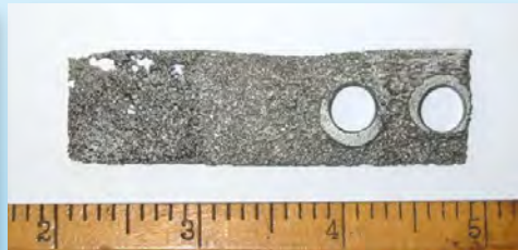
Corrosion coupons are used to assess general corrosion rates and microbial growth
